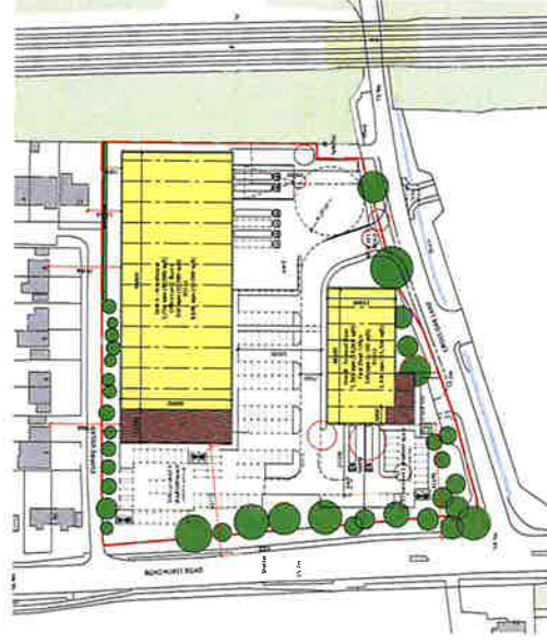
09 July 2021: TWO BUILDINGS - 2 UNITS, NEW ACCESS ROAD, CLOSER TO EMPIRE VILLAS BOUNDARY RETAIN MORE TO CROSS OAK LANE, CAR PARK ADJACENT EMPIRE VILLAS
